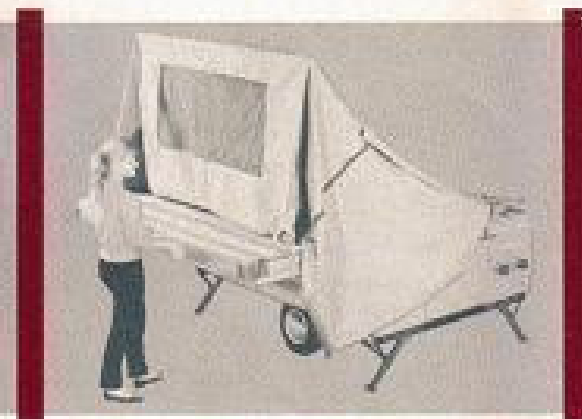
Travelling cover is removed, bow system raised and beds pulled out to begin assembly.
